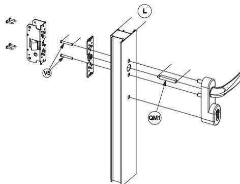
Measure the door lock stile thickness (L in diagram above). Then adjust spindle (QM1) length and V5 machine screw using following formula:
