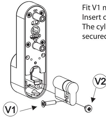
Fit V1 machine screw into cylinder body. Insert cylinder into rear of housing. The cylinder and V1 screw can now be secured with V2 pan head machine screw.
