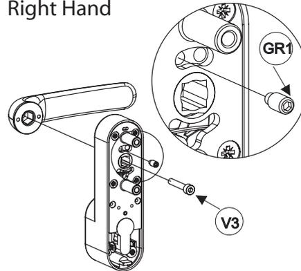
Using the diagram, left, secure lever to housing using V3 socket cap screw.
