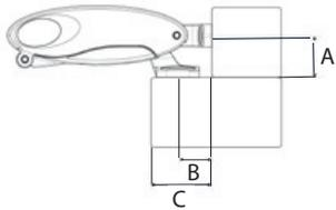
A = Fixing centre to frame 25mm
