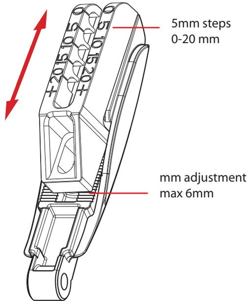
Open the Duoflex opener, loosen off the screw on base of opener using a 3mm allen key. This will release the top part of the bottom bracket allowing the arm to be inserted into appropriate slot. The top bracket can also be moved along the mm increments for finer adjustment. Once required step is achieved the screw at the bottom can be tightened back up and folding opener fitted to window.
