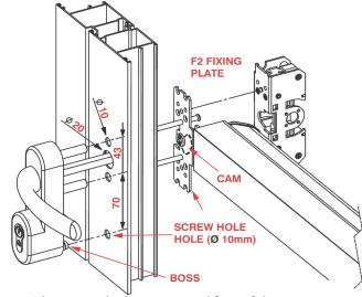
Fit outside access device to external face of door.
