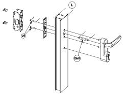
Measure the door lock stile thickness (L in diagram above). Then adjust spindle (QM1) length and V5 machine screw using following formula: Spindle Length = L + 13mmV5 machine screw = L - 10mm TRIM SPINDLE AT THE SOUARE END ONLY
