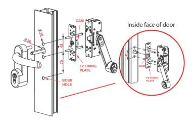
Fit outside access device to external face of door.
