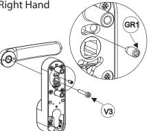
Using the diagram, left, secure lever to housing using V3 socket cap screw.
