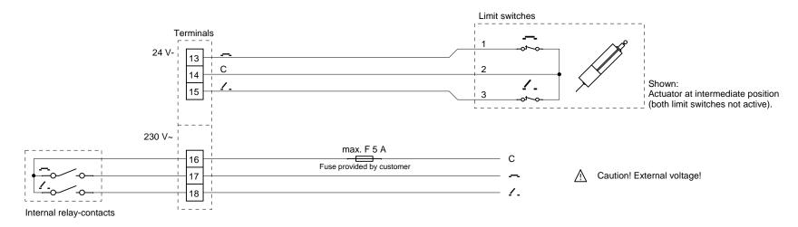
The relay contact "Closed" will be closed, if all limit switches for the position "Closed" are activated. The relay contact "Open" will be closed, if all limit switches for the position "Open" are activated. At intermediate positions both contacts are opened.
