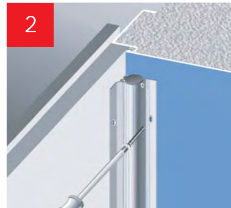
2 Fix with screws provided
