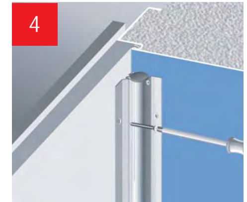
4 Fix with screws provided
